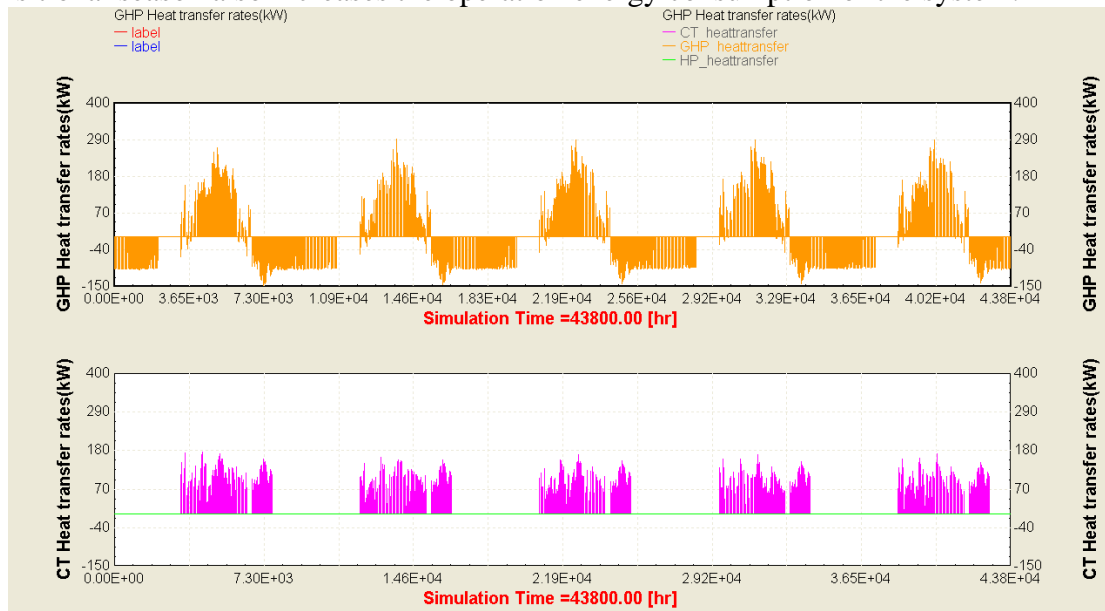
Fig.5. Hourly acquired and released heat amount of buried pipe and cooling tower (strategy 1 and 5, 5th to 10th years)
